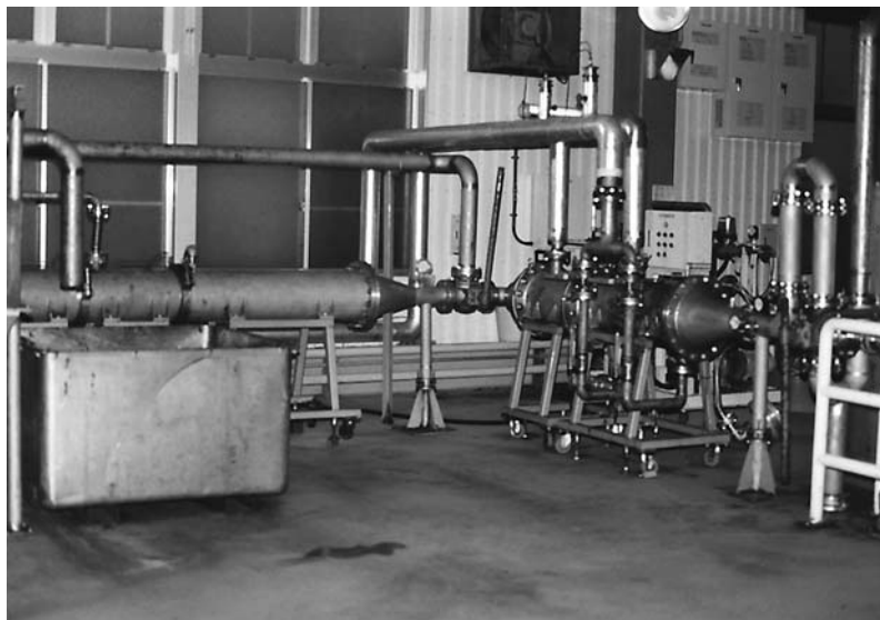
Figure 13 Pasteurization of miso with a continuous pasteurizer. (Courtesy of Sendai Miso Shoyu Co. Ltd.)
