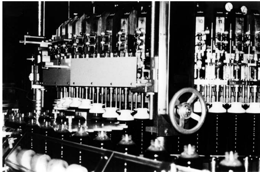
Figure 47 Filling of soy sauce into 1-L plastic bottles. (Courtesy of the Kikkoman Corporation.)
