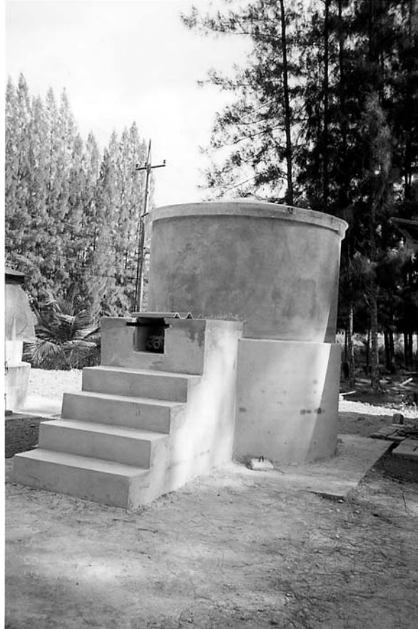
Figure 4 After the fermentation period, fish sauce is transferred to a nearby concrete storage tank to age before bottling. This practice is for small- to medium-scale production.
