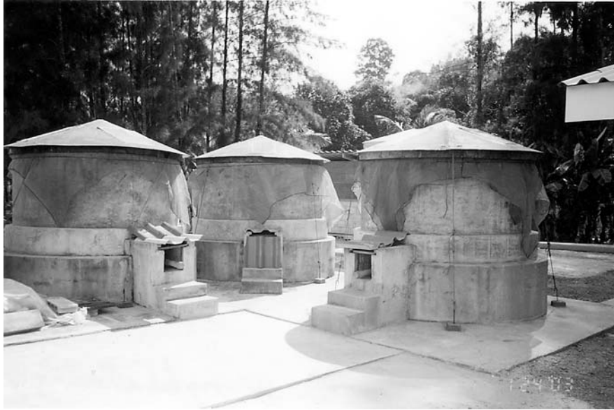
Figure 3 Fish and salt are mixed (3 : 1 ratio, w/w) and put in concrete tanks (2.5-ton capacity) covered with a nylon net and fiberglass lid for fermentation. After 12–15 months, fish sauce is filtered a charcoal bed packed at the bottom of the tank and the clear sauce is collected from the pipe at the opening channel.
