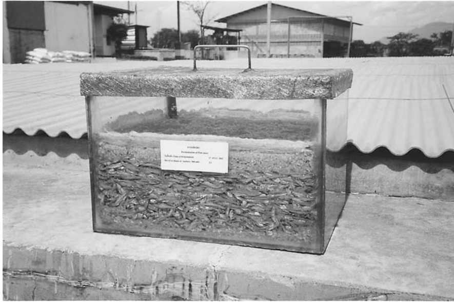
Figure 7 Fermentation pool model showing the mixture of fish and salt in the pool. The top layer is salt. (Courtesy of Pichai Fish Sauce Co., Ltd.)
