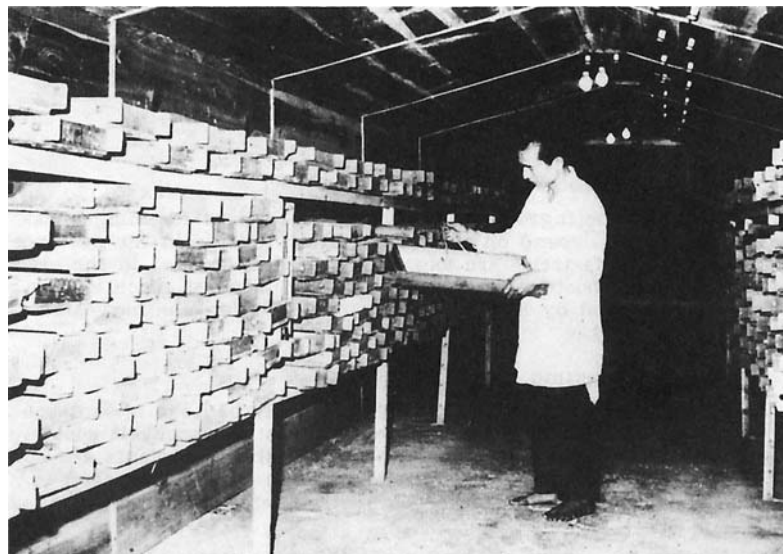
Figure 14 Koji chamber for indigenous miso manufacture. A craftsman is measuring the temperature of koji on a koji tray. (From Ref. 10.)
