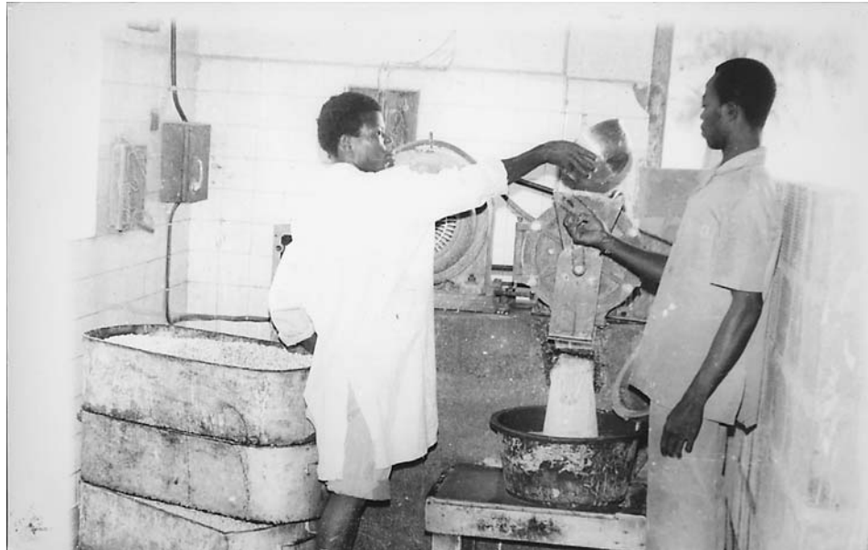
Figure 9 Wet milling of softened fermenting grain in a Sprout Waldron electric disk mill. (Courtesy of the Federal Institute of Industrial Research, Oshodi, Lagos, Nigeria.)
