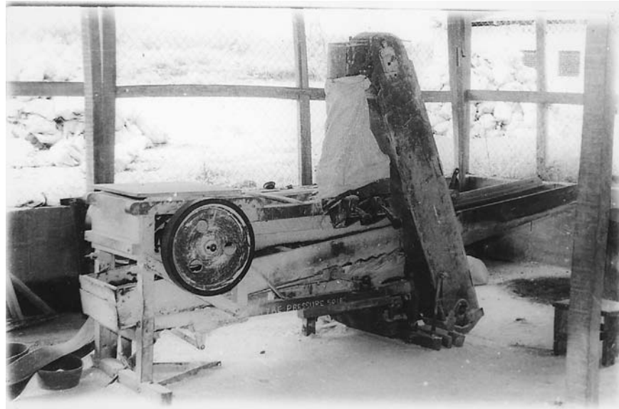
Figure 24 Commercial industrial gari production. Deck sifter grading of milled gari granules. (Courtesy of the Federal Institute of Industrial Research, Oshodi, Lagos, Nigeria.)
