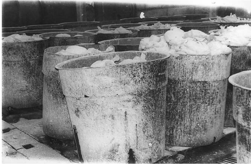
Figure 14 Commercial industrial gari production. Bagged pulped roots fermenting in plastic open-bottom modern vats. (Courtesy of the Federal Institute of Industrial Research, Oshodi, Lagos, Nigeria.)
