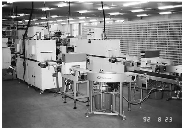
Figure 23 Packaging room and cup wrapping machine. (Courtesy of Suzuyo Kogyo Co. Ltd.)
