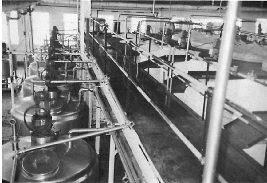
Figure 11 Transfer of maize meal porridge (substrate) to stainless-steel or fiberglass bioreactors.
