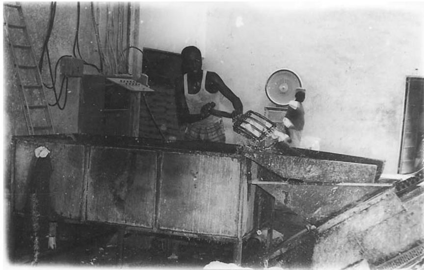
Figure 10 Commercial industrial gari production. Peeled cassava tubers being transferred into wash tanks. (Courtesy of the Federal Institute of Industrial Research, Oshodi, Lagos, Nigeria.)
