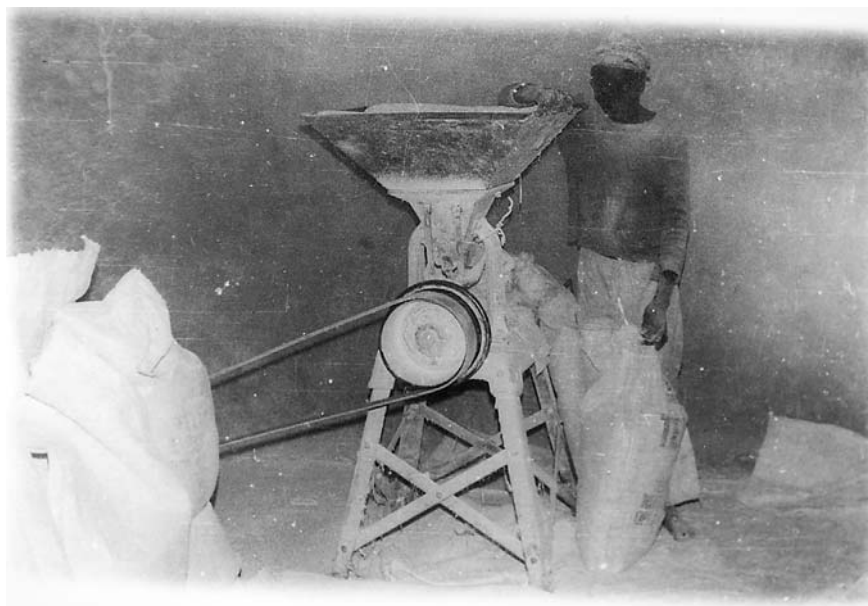
Figure 23 Commercial industrial gari production. Milling of course gari. (Courtesy of the Federal Institute of Industrial Research, Oshodi, Lagos, Nigeria.)
