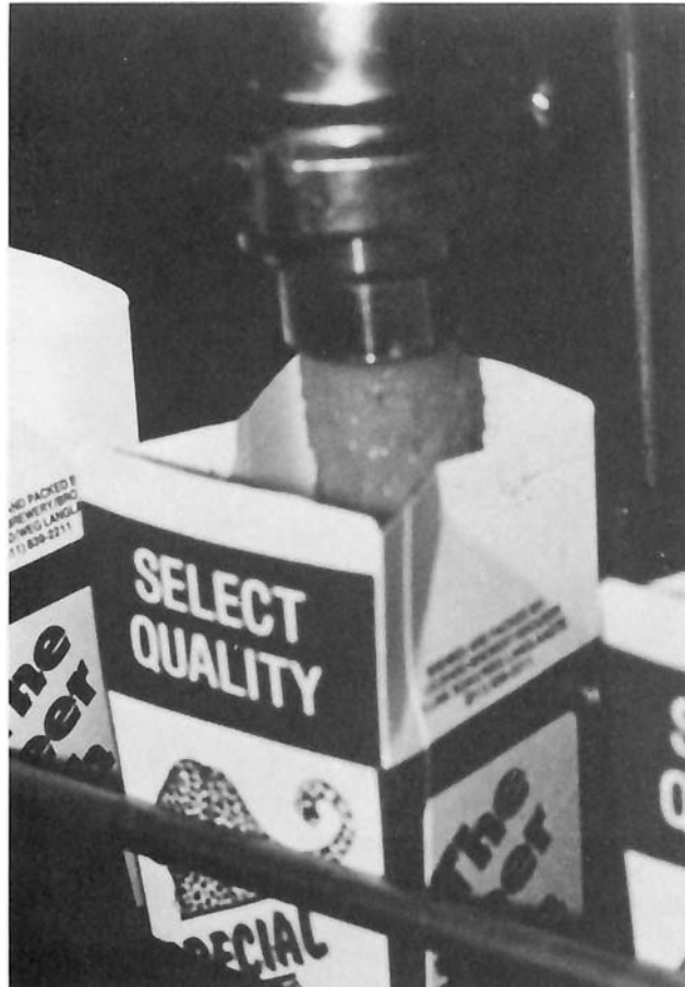
Figure 39 One-liter wax paper carton being filled with sorghum beer (South Africa). (Courtesy of the Sorghum Beer Unit of the Council for Scientific and Industrial Research, Pretoria.)
