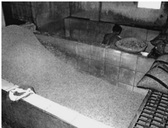
Figure 16 Soaking soybean cotyledons after dry dehulling.
