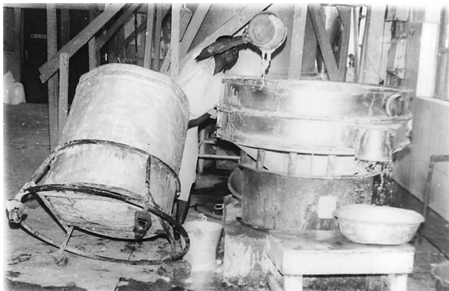
Figure 10 Sieving of grains slurry in a vibrating sieve (vibroscreen) having a 310- \mu\text{m} mesh aperture. (Courtesy of the Federal Institute of Industrial Research, Oshodi, Lagos, Nigeria.)
