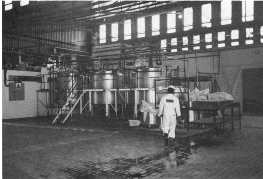
Figure 10 Cooking of maize meal porridge in stainless-steel vessels at 85–90°C for 20–30 min.
