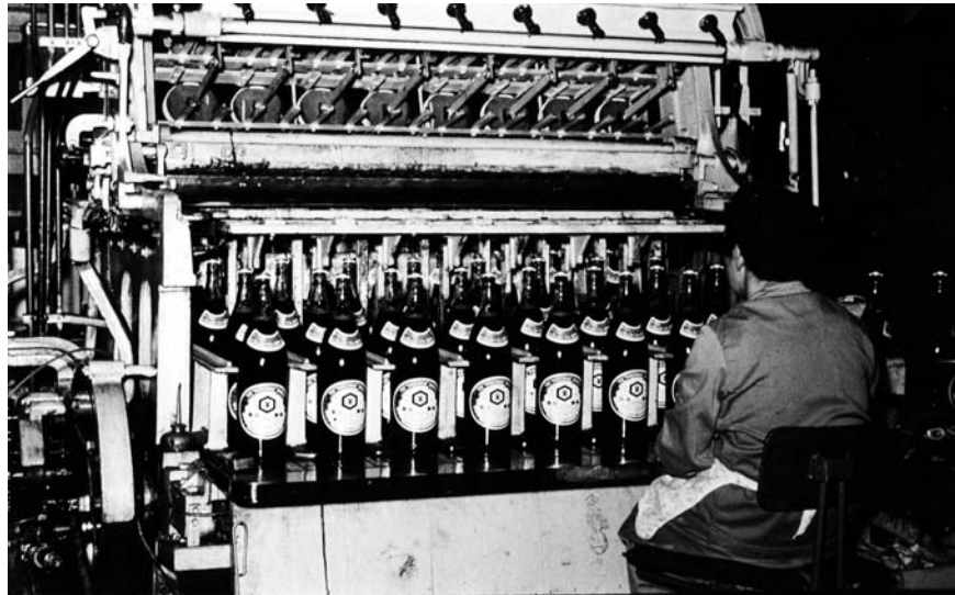
Figure 46 Filling of soy sauce into 2-L glass bottles. (Courtesy of the Kikkoman Corporation.)
