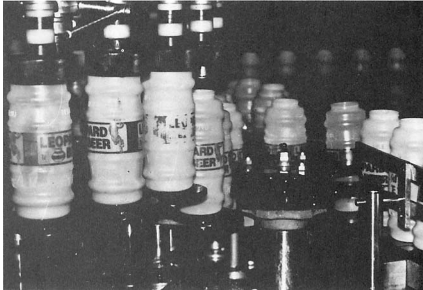
Figure 40 One-liter high-density polyethylene containers being filled on a low-vacuum filling machine (South Africa). (Courtesy of the Sorghum Beer Unit of the Council for Scientific and Industrial Research, Pretoria.)
